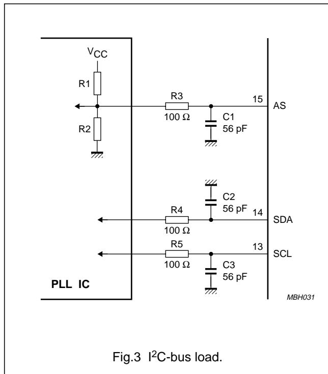
Fig.3 I<sup>2</sup>C-bus load.
